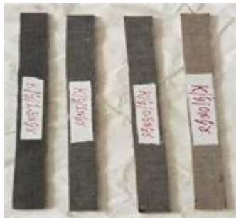
Fig 3: Before Tensile Test specimens.
