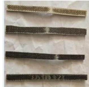
Fig 4: After Tensile Test specimens
