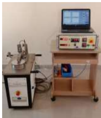
Fig 3: Experimental Setup of Pin and Disc
