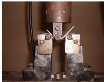
Fig 13: Loading arrangement of the specimens for flexural test
