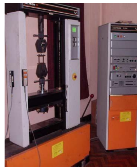
Fig 10: Experimental set up of specimen for tensile strength test
