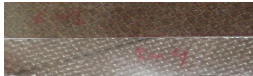
Fig 8: Tensile test specimen of Jute/Hemp/glass fiber reinforced epoxy composites(photography)
