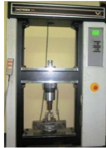
Fig 12: Experimental setup of the specimens for flexural test
