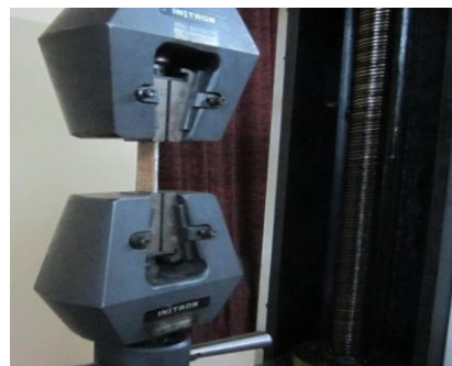
Fig 11: Loading arrangement of specimen for tensile strength test
