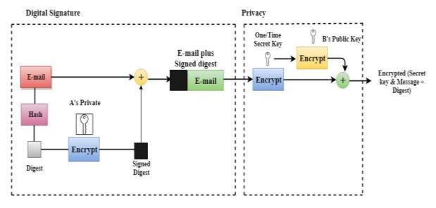
Following are the steps taken to show how PGP uses hashing and a combination of three keys to generate the original message:
