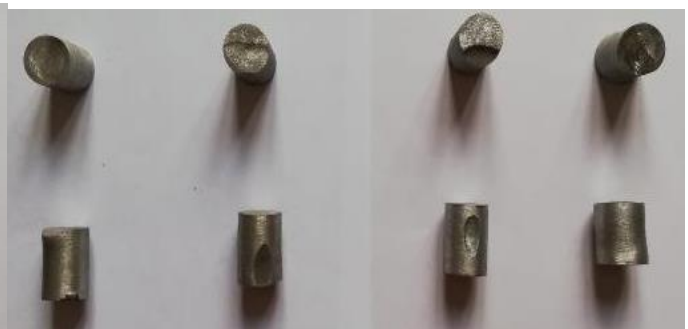
Fig: Compression tested specimen
