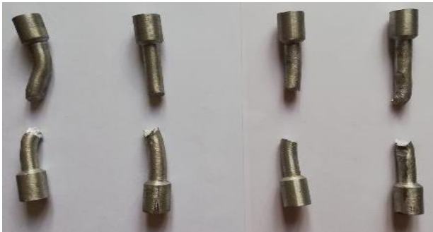
Fig: Tensile tested specimen
