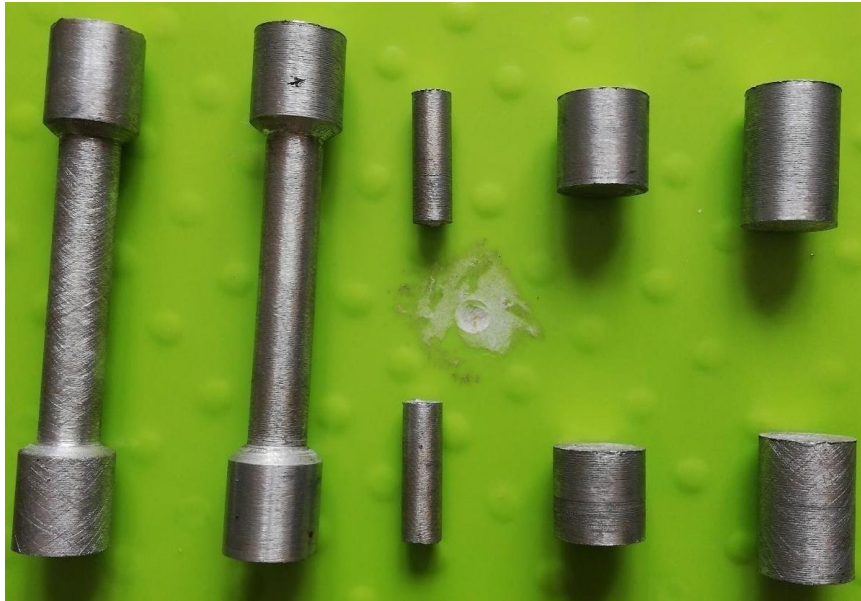
Fig: Specimens machined according to ASTM standards
