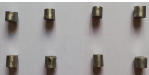
Fig: Brinell Hardness tested specimen
