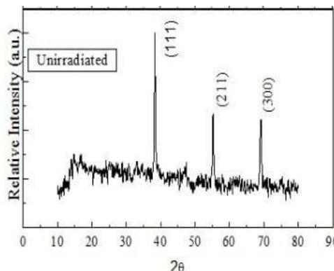
FIGURE 3.1 XRD of Barium Zirconate ceramic
