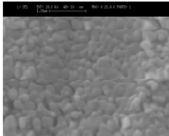
**FIGURE 3.2** SEM micrographs of UI, Barium Zirconate
