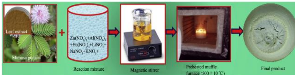
Fig.3. Schematic diagram of combustion synthesis of ZAE:M^+ ( M^+ = K^+, Na^+ and Li^+ )
