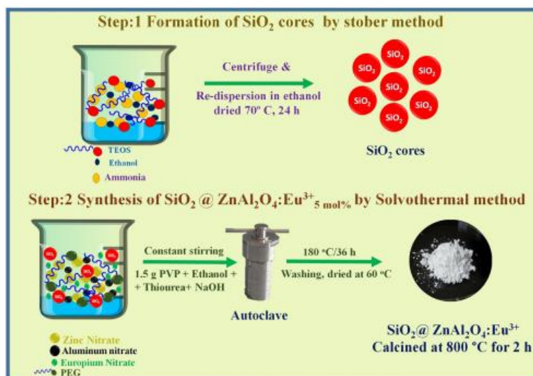
Fig.2 Schematic illustration for the formation process of SiO_2 core and core-shell SiO_2@ZnAl_2O_4:Eu^{3+}
