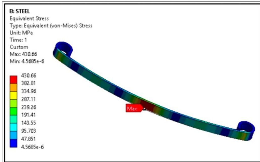
Fig. 2 Equivalent Stress-Steel Spring
