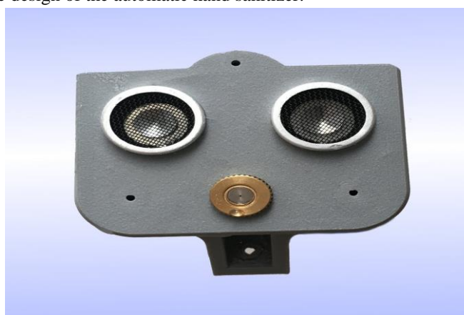
Figure 9. Ultrasonic Sensor and Nozzle Assembly
