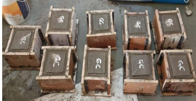
Fig. 9. Ferrocement jacketed GCC cubes.
