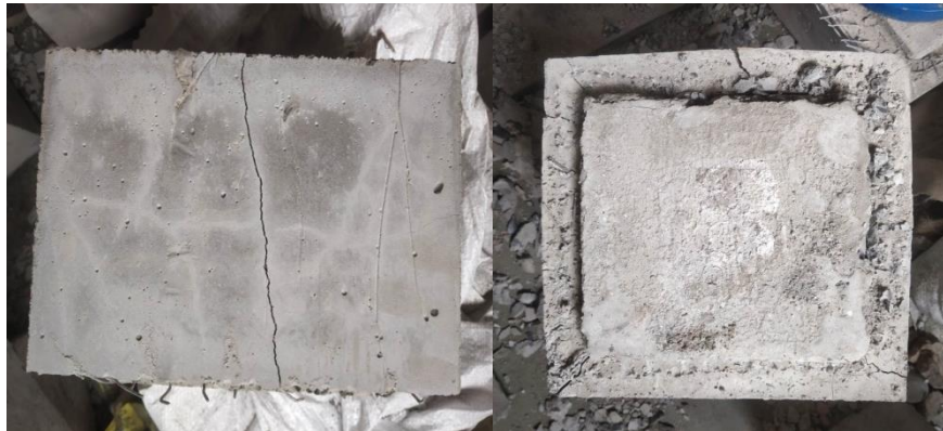
Fig. 10. Cracks in PCC ferrocement jacketed cubes.
