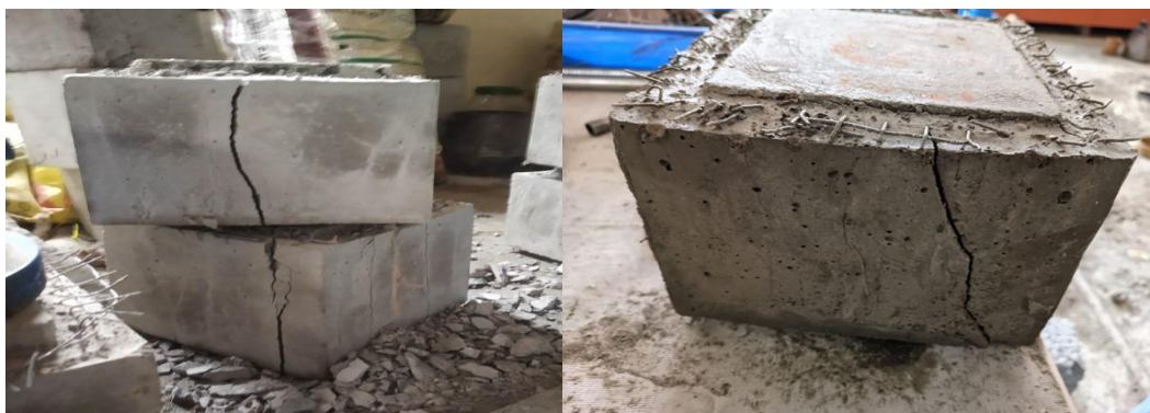
Fig. 11. Cracks in GCC ferrocement jacketed cubes.
