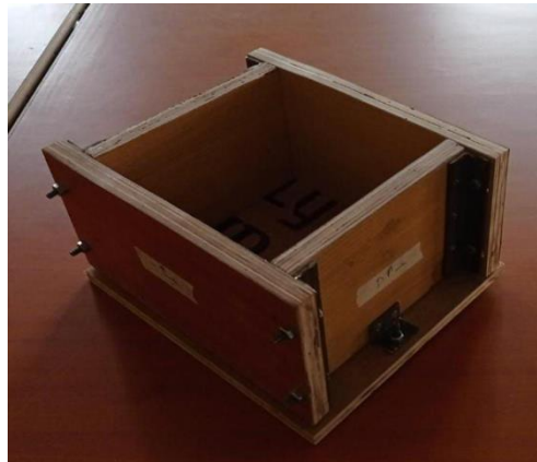
Fig. 2. Mould for ferrocement.
