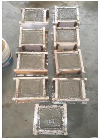
Fig. 6. Ferrocement jacketed PCC cubes
