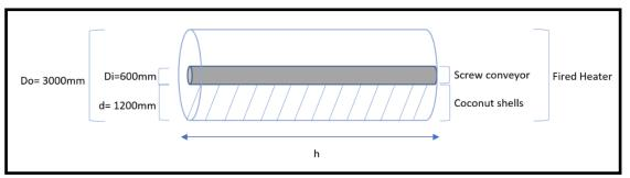
The following data is obtained and assumed to calculate the dimensions of the equipment. To find length of fired heater according to volume of coconut shells processed:
