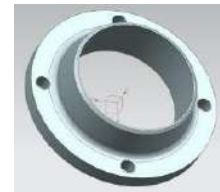
Fig3.09: 3D sketch of Nozzle 3
