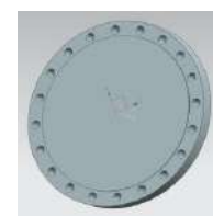
Fig3.12: 3D sketch of Manhole
