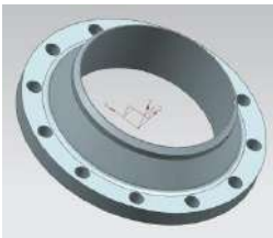
Fig3.07: 3D sketch of Nozzle 8 in NX in NX
