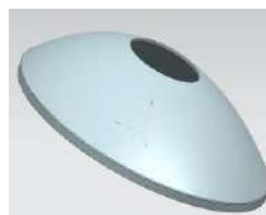
Fig3.11: 3D sketch of Dishend 2 in NX
