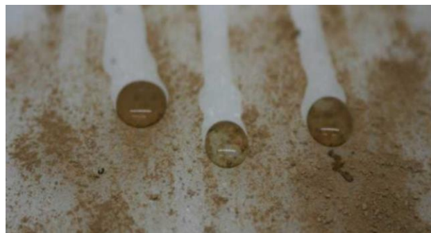
Fig4: Picture depicting rolling down of water droplets carrying dust particles on a superhydrophobic surface[33].
