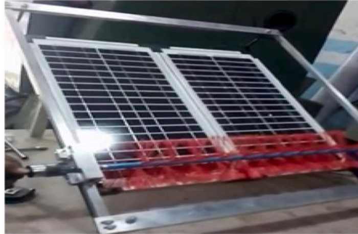
Fig9: Brush cleaning system
