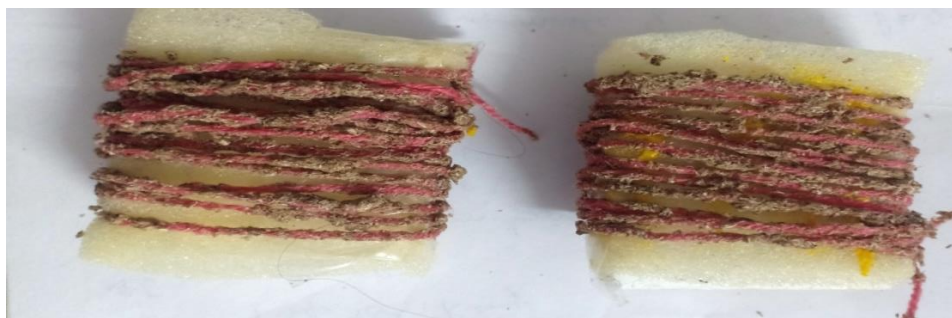
Photo showing coating of sawdust paste on wool wrapped on synthetic sponge.
