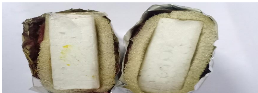
Photo- showing –XPS- Polystyrene – sawdust- wool model
