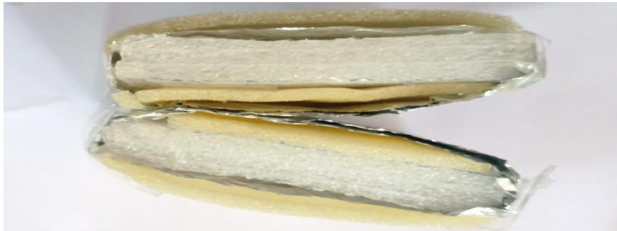
Photo showing – Polyurethane Foam-Aluminium foil thermal insulator.
