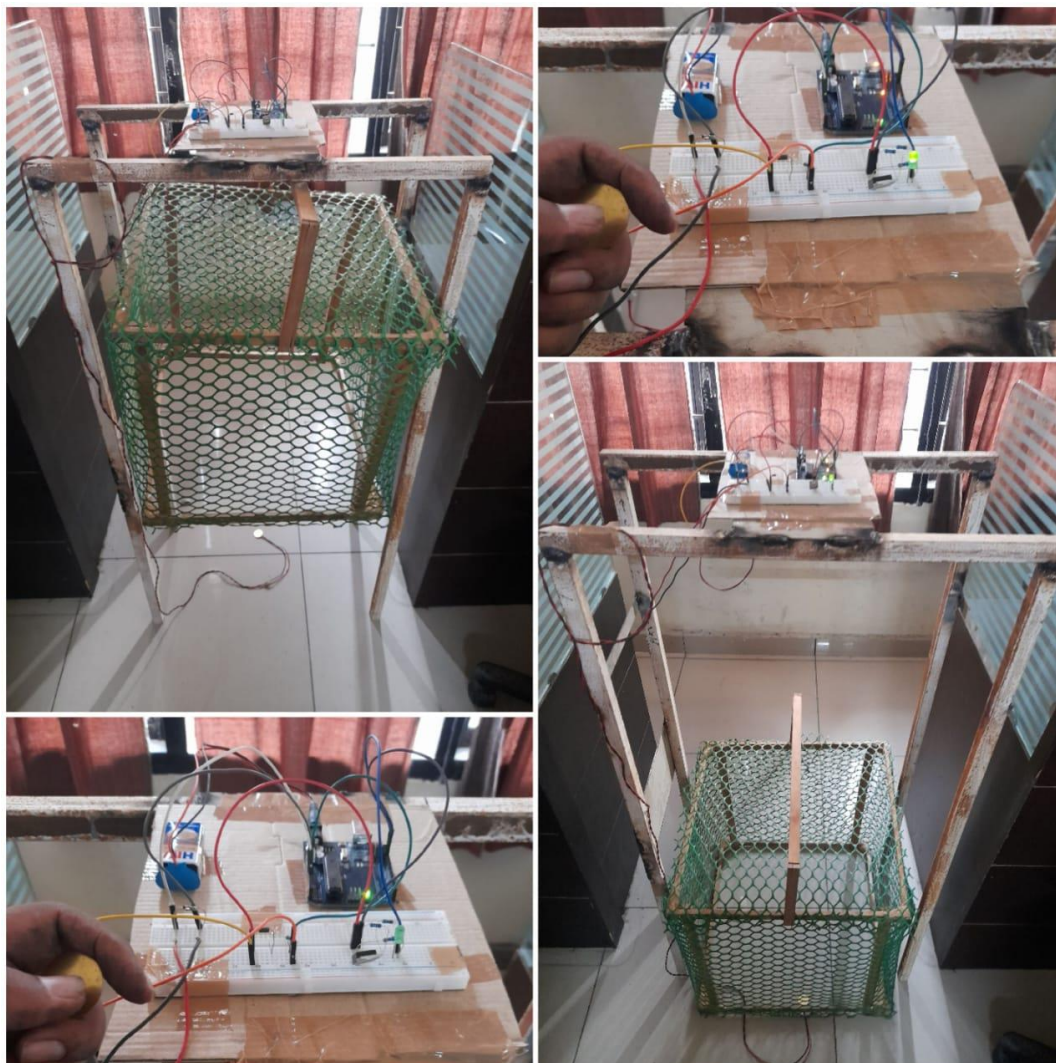
Fig. 4. Pressure activated wild boar trap
