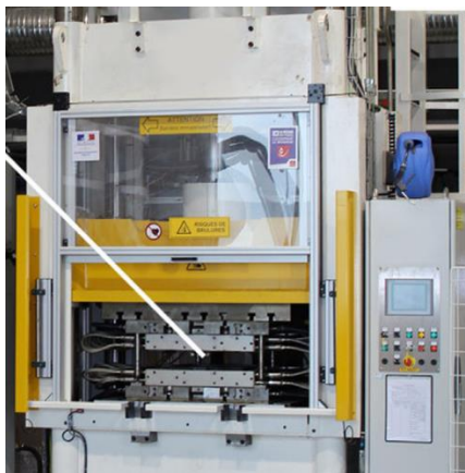
Figure 3: Machining setup of Compression molding process
