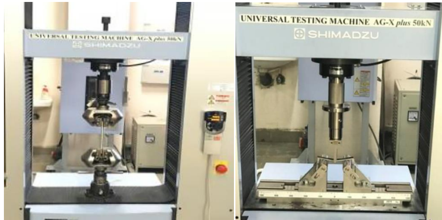
Figure 4: Testing Equipment setup of Tensile and Flexural test
