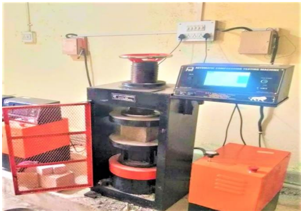
Fig.5 Compressive Strength Testing Machine
