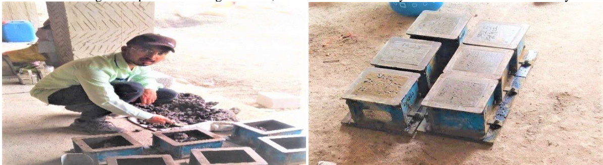
Fig.3 Casting Of Cubes
