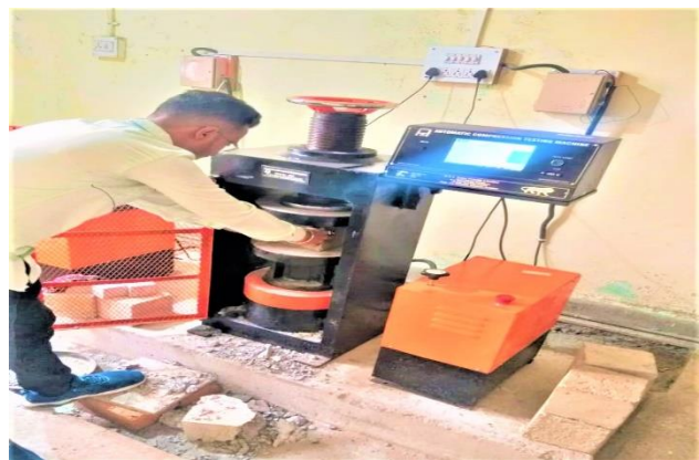
Fig.6 Compressive Strength of Cubes
