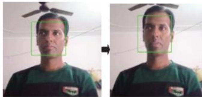
Fig. 5. Facial landmarks detection and ROI selection
