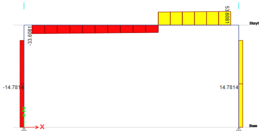
Fig 5.1.3: shear force diagram analyzed by E-tabs
