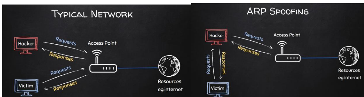
Figure 2: The typical network diagram shows how the ARP-Disguising attack occurs
