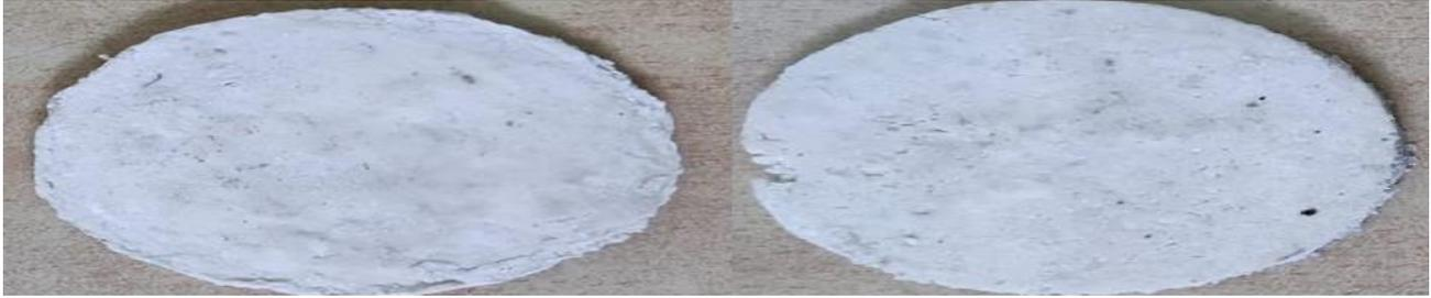
Fig 1. Prepared on composite membrane of 4% TiO<sub>2</sub> and 4% ZrO<sub>2</sub>
