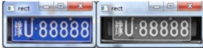
Figure 3 shows the results of the first. method one, and method two the licence plate location is skewed in the second type of image.
