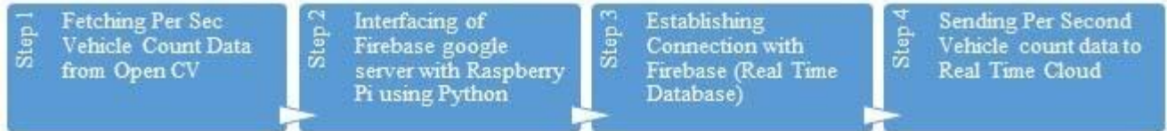
Fig. 2: Systematic flow diagram to illustrate the image processing operations for obtaining the count of the present vehicles
