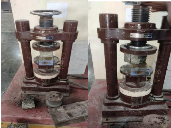
Fig 3: (a) Compression strength test
