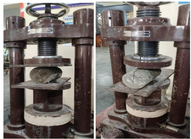
(b) Split tensile strength test
