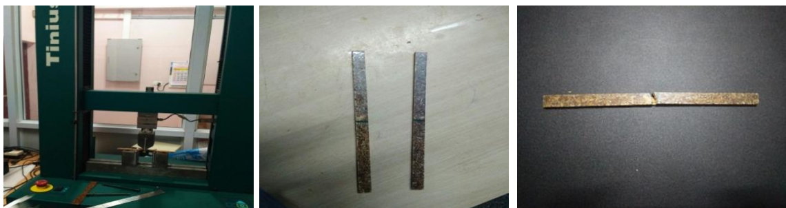
Figure4: (a) Specimen loaded in UTM (b) Specimen before flexural test (c) Specimen after flexural test.
