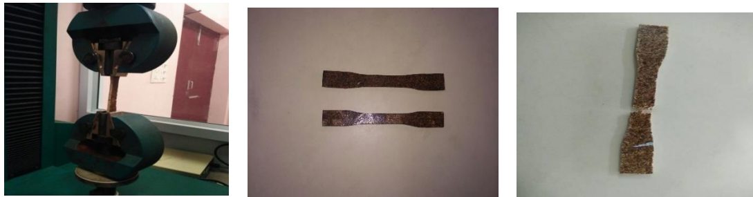
Figure 3: (a) Specimen loaded in UTM machine (b) Specimen before tensile test (c) Specimen after tensile test.
