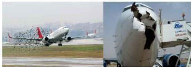
Fig 1: An example of Bird Strike and damage to the plane
