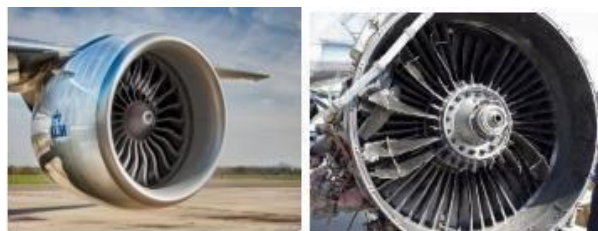
Fig 2: Normal Jet Engine and Jet Engine after Bird Strike
