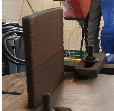
Figure 3. Image of SS308L wall component by using CMT process.
