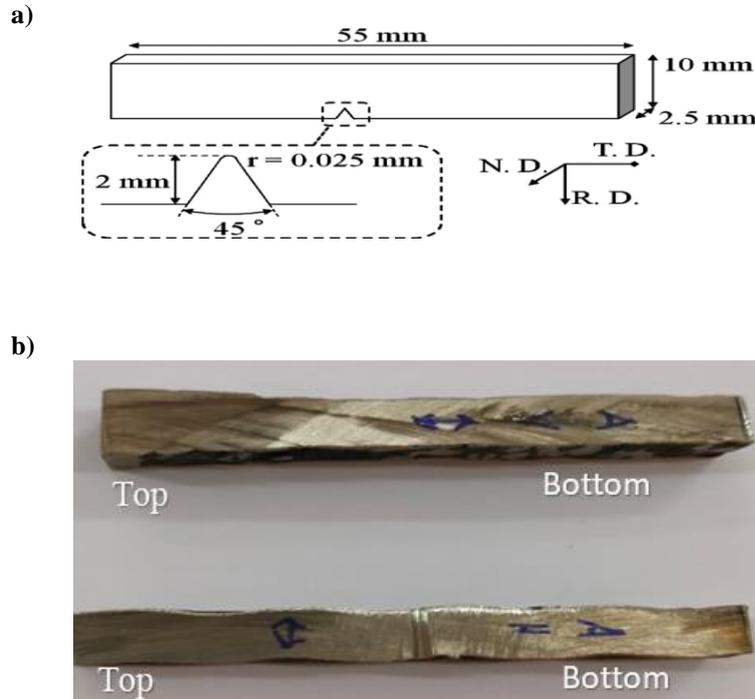
Figure 5. a) Dimension of the impact specimen b) image of the Impact specimen
