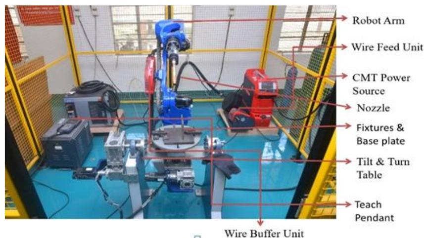
**Figure 1. GMAW-CMT WAAM setup used to fabricate SS308L wall component**
