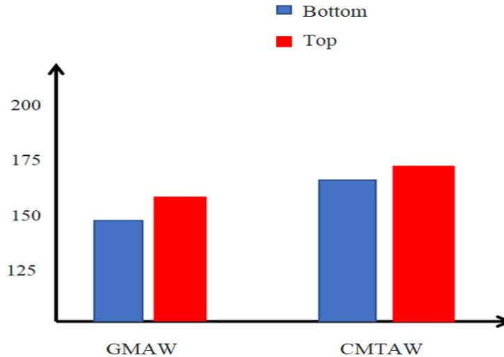
**Figure 7. Vickers micro hardness distribution on the surface**
