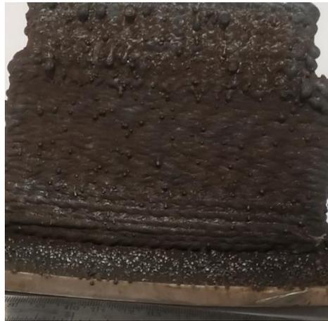
**Figure 2. Image of SS308L wall component by using the GMAW process**
