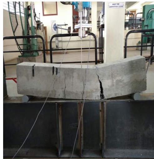
Fig: Failure of B1
