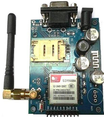
**Fig.No.2 - GSM Module****Microcontroller**
