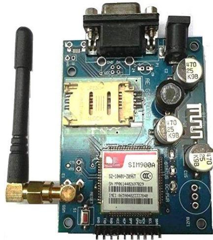
**Fig.No.2 - GSM Module****Microcontroller**
