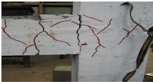
Fig. 9 Comparison of joint failure between A) Test specimen and B) Simulated model of specimen - 1
