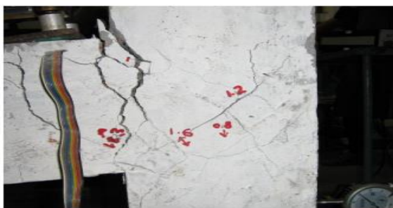
Fig. 13 Comparison of joint failure between A) Test specimen and B) Simulated model of specimen -2
