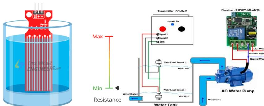
Fig. 2 Schematic diagram of the proposed model using AI sensors
