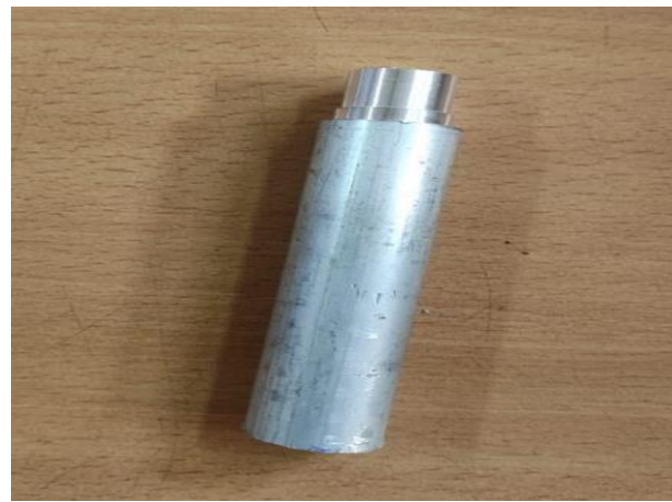
Fig. 4 Aluminium workpiece after turning operation
