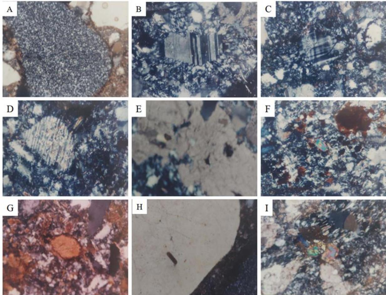
**Fig. 4:** (A) Photomicrographs of Chert grain in greywackes. (B) Plagioclase feldspar in greywackes. (C) Microcline Feldspar. (D) Plagioclase grain undergone saussurite. (E) Carbonates in greywackes. (F) Zircon in greywackes. (G) Sphene in greywackes. (H) Zircon and Apatite. (I) Epidote in greywackes.
