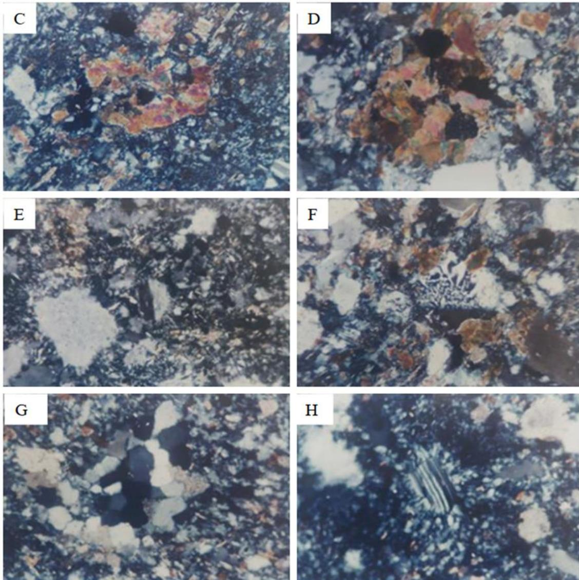
**Fig. 3:** (C) Photomicrograph shows poorly sorted nature of grains. (D) Photomicrograph shows a cluster of Biotite grains in greywackes. (E) Photomicrograph shows presence of Orthoclase. (F) Photomicrograph shows presence of igneous rock fragments. (G) Photomicrograph shows polycrystalline quartz. (H) Photomicrograph shows “Chevaux-de-frise” plagioclase feldspar.
