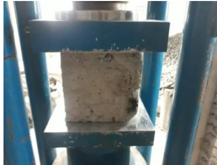
fig 4 : Compression test of concrete cube
