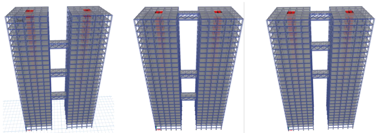
Figure 14 Three skybridge at a time on the 14 th & 7 th & 21 st floor, 14 th & 7 th & 28 th floor, 14 th & 21 st & 28 th floor
