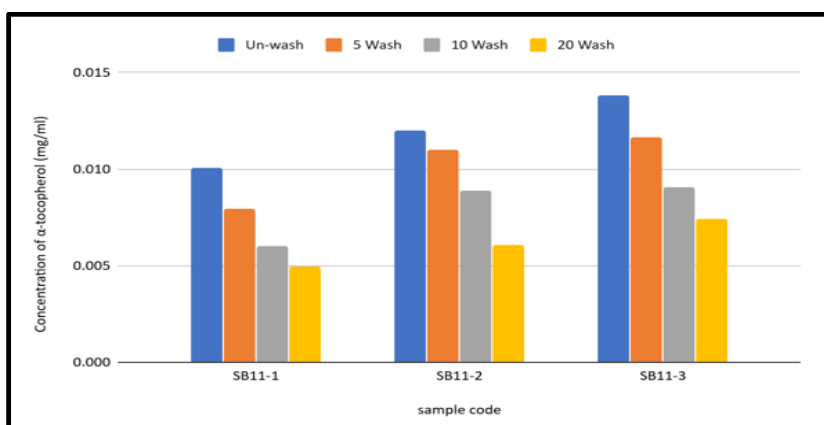
Figure 13: Release of \alpha -tocopherol from sericin/ \beta -cyclodextrin treated cotton fabric samples at different washing cycle.
