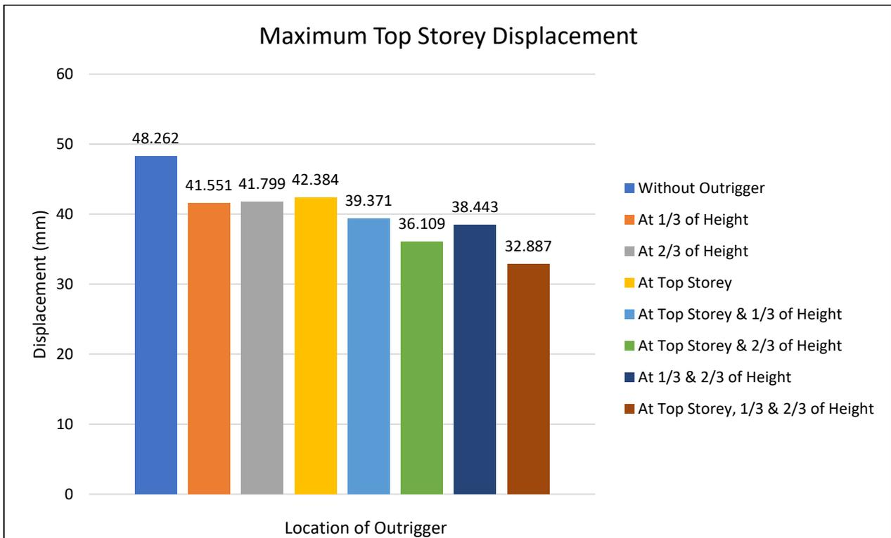
Figure 29 Maximum Top Storey Displacement in RS-X & Y Direction (Response Spectrum)
