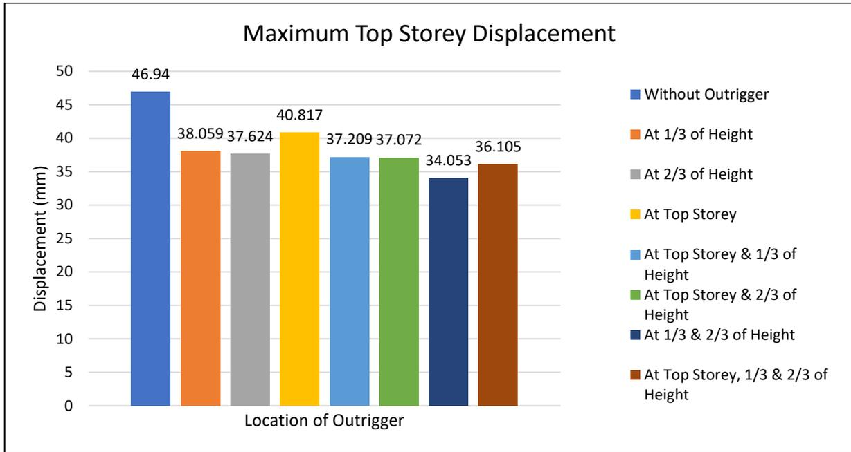
Figure 14 Maximum Top Storey Displacement in RS-X & Y Direction (Response Spectrum)
