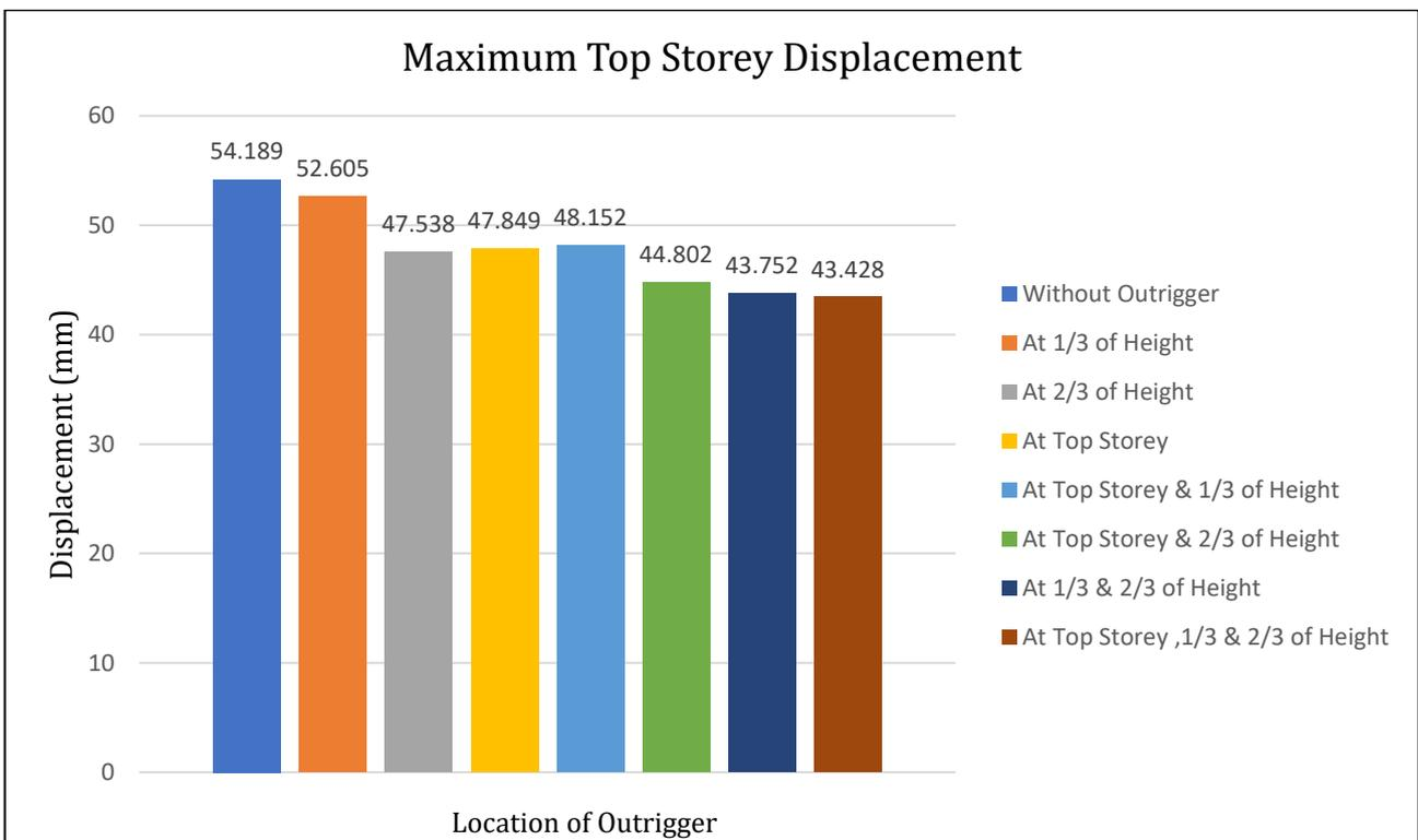
Figure 27 Maximum Top Story Displacement in EQ-X & Y Direction (Earthquake Static)
