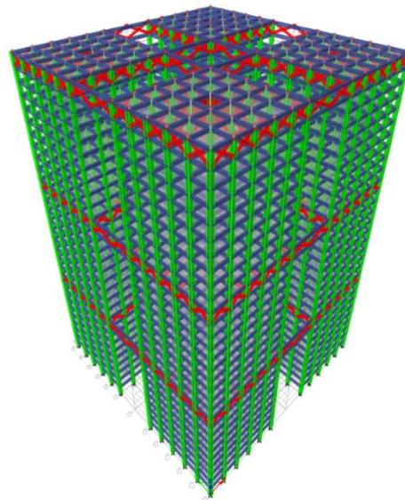
Figure 7 3D view of G+29 Belt-truss outrigger building
