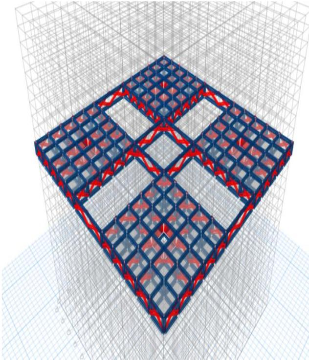
Figure 4 Belt-truss outrigger system
