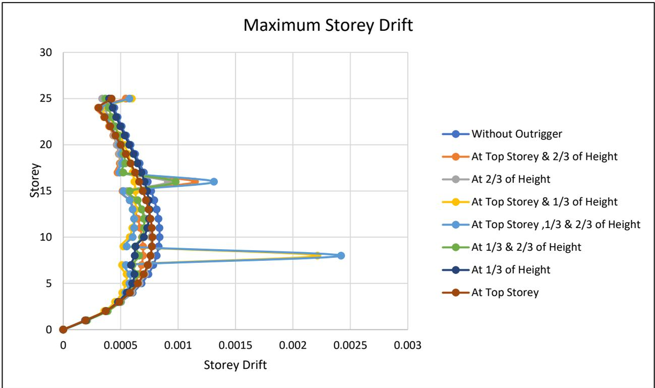
Figure 20 Maximum Story Drift in RS-X & Y Direction (Response Spectrum)
