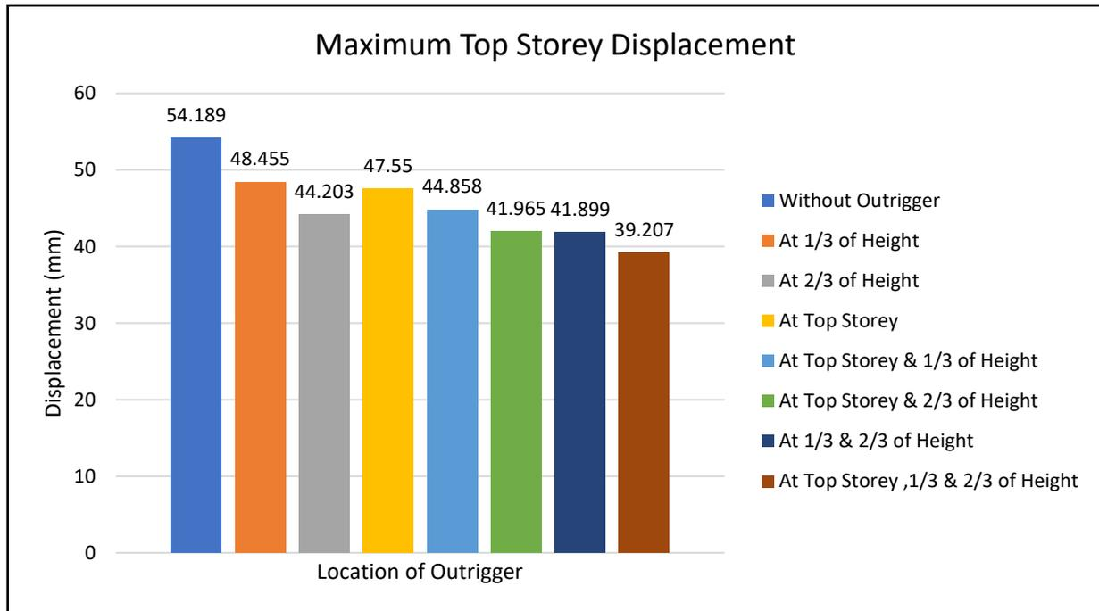
Figure 22 Maximum Top Story Displacement in EQ-X & Y Direction (Earthquake Static)
