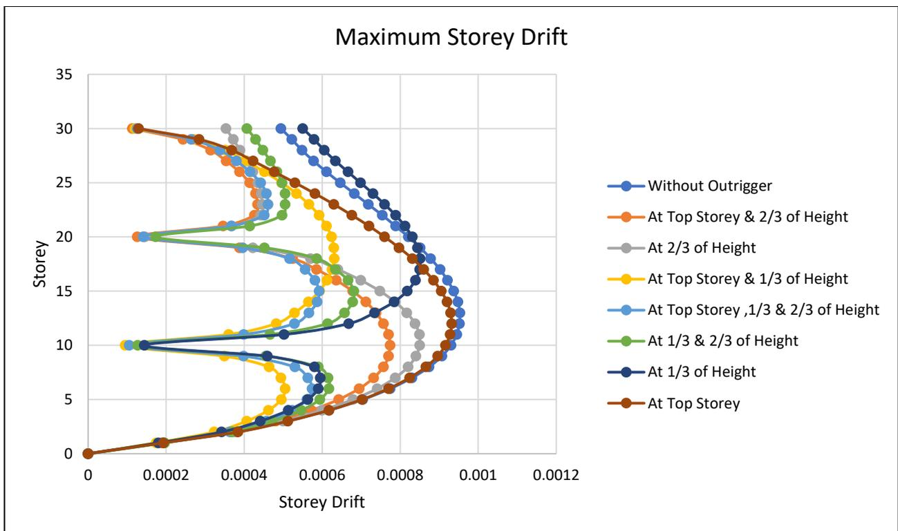
Figure 35 Maximum Storey Drift in RS-X & Y Direction (Response Spectrum)
