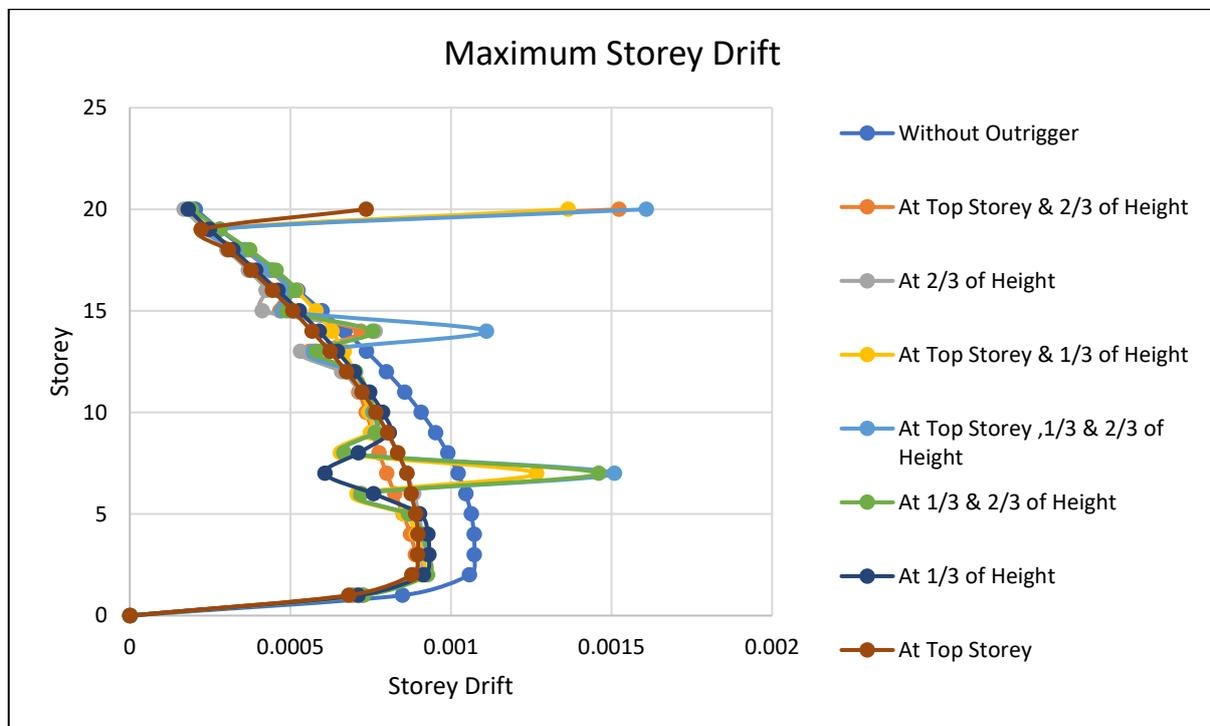
Figure 15 Maximum Storey Drift in RS-X & Y Direction (Response Spectrum)
