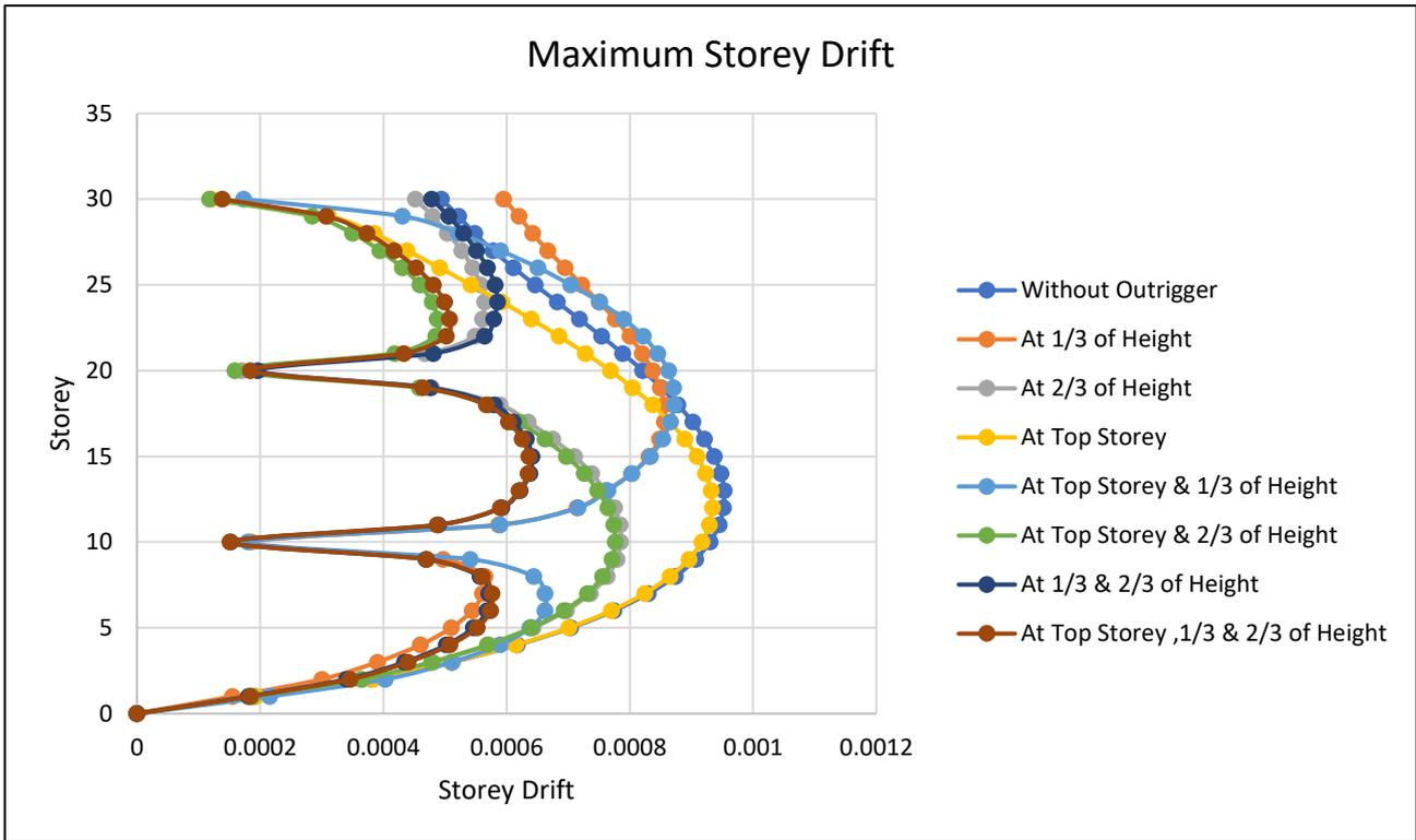
Figure 40 Maximum Story Drift in RS-X & Y Direction (Response Spectrum)
