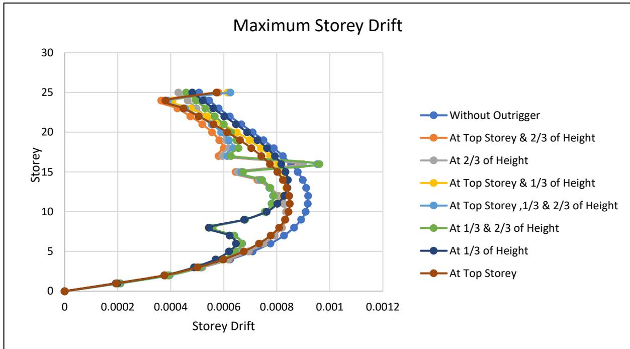
Figure 18 Maximum Storey Drift in EQ-X & Y Direction (Earthquake Static)
