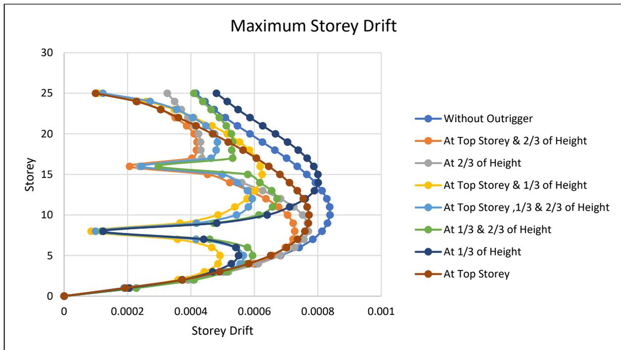
Figure 25 Maximum Storey Drift in RS-X & Y Direction (Response Spectrum)
