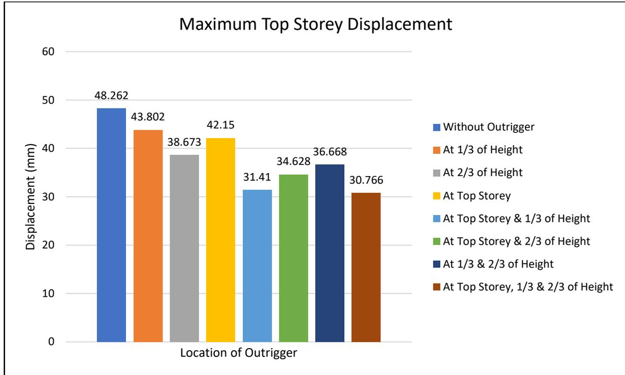
Figure 24 Maximum Top Story Displacement in RS-X & Y Direction (Response Spectrum)
