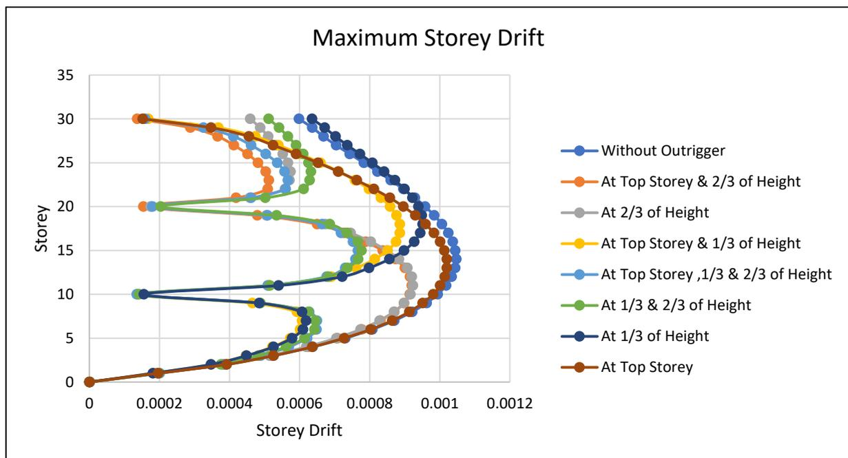
Figure 33 Maximum Storey Drift in EQ-X & Y Direction (Earthquake Static)
