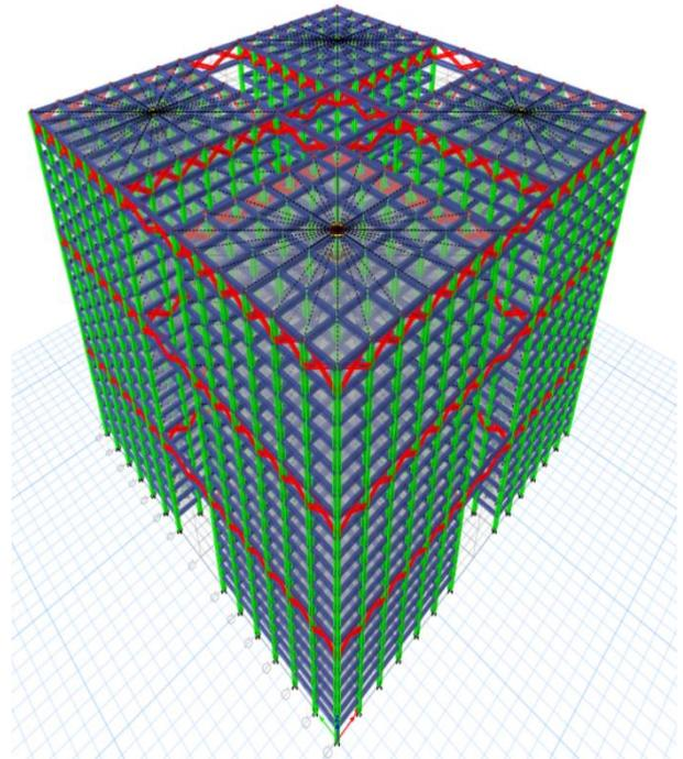
Figure 5 3D view of G+19 Belt-truss building
