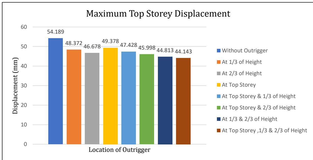
Figure 17 Maximum Top Story Displacement in EQ-X & Y Direction (Earthquake Static)
