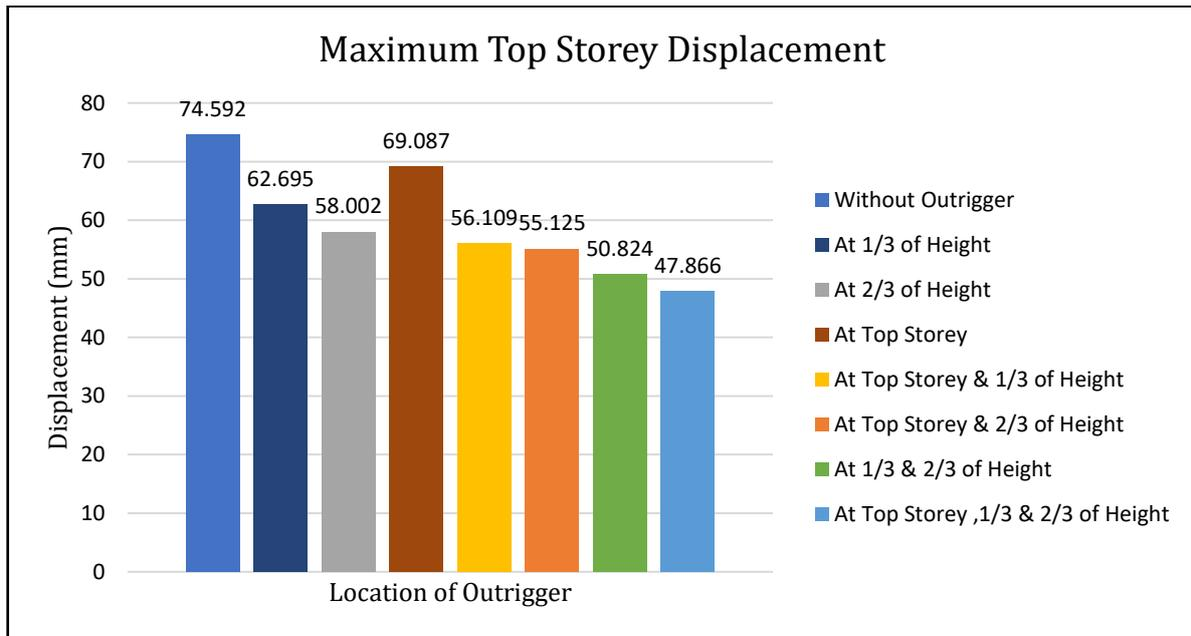
Figure 32 Maximum Top Story Displacement in EQ-X & Y Direction (Earthquake Static)
