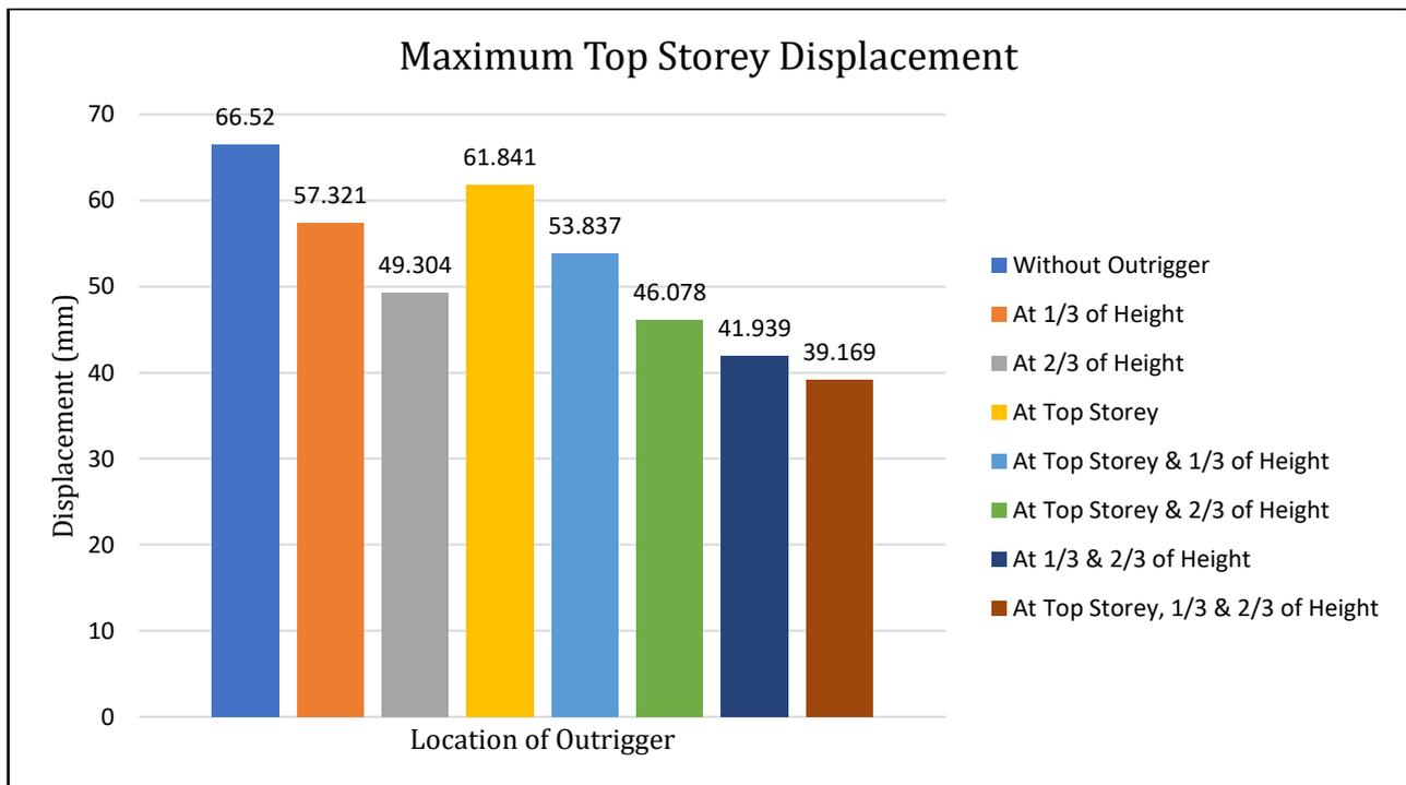
Figure 39 Maximum Top Storey Displacement in RS-X & Y Direction (Response Spectrum)
