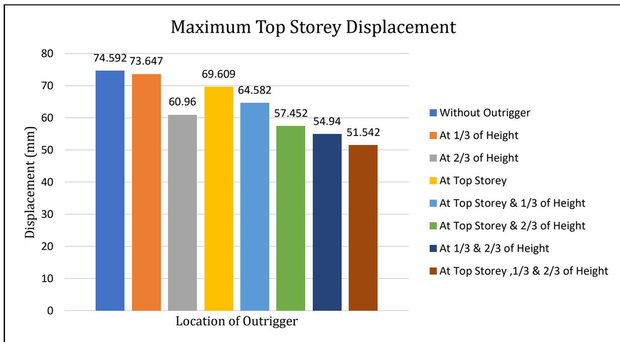
Figure 37 Maximum Top Storey Displacement in EQ-X & Y Direction (Earthquake Static)
