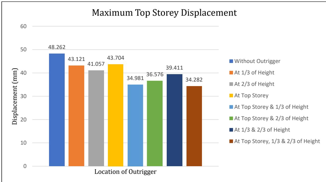
Figure 19 Maximum Top Storey Displacement in RS-X & Y Direction (Response Spectrum)
