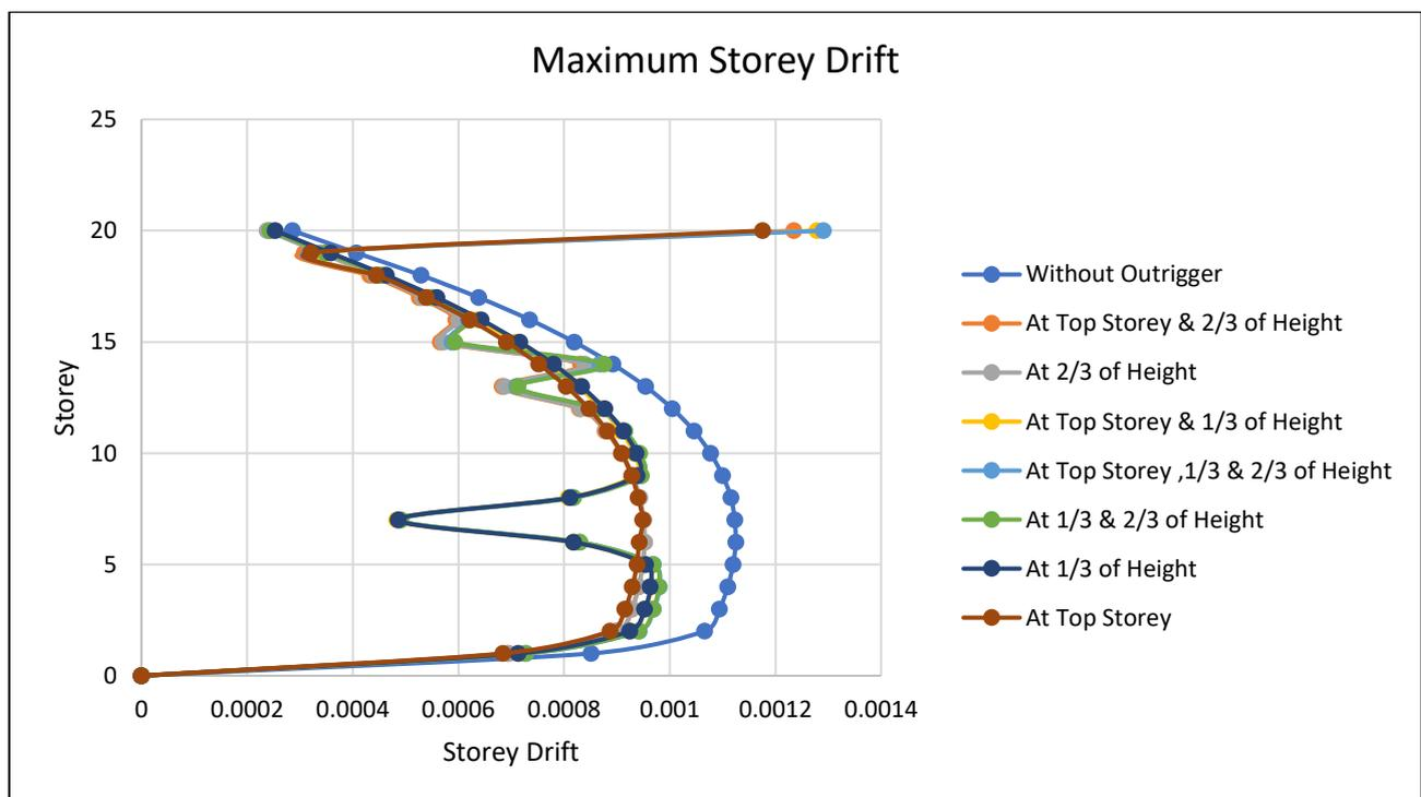
Figure 13 Maximum Storey Drift in EQ-X & Y Direction (Earthquake Static)
