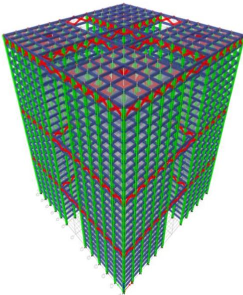
Figure 6 3D view of G+24 Belt-truss outrigger building
