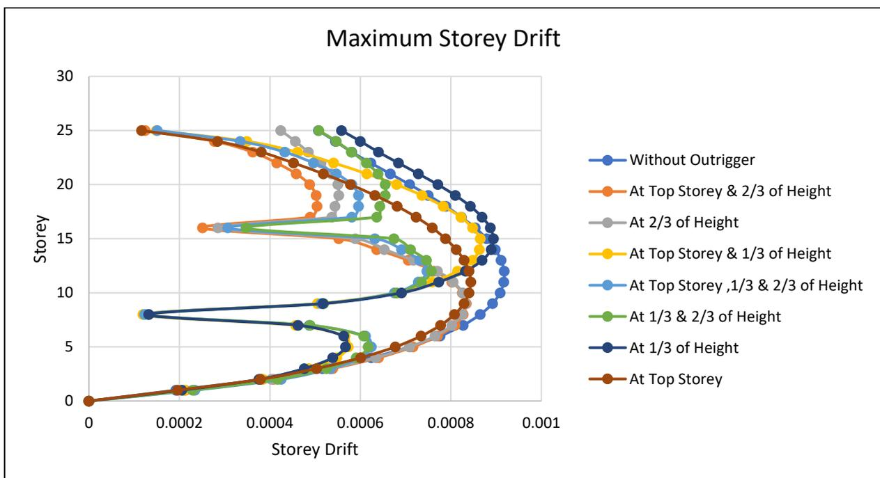
Figure 23 Maximum Storey Drift in EQ-X & Y Direction (Earthquake Static)
