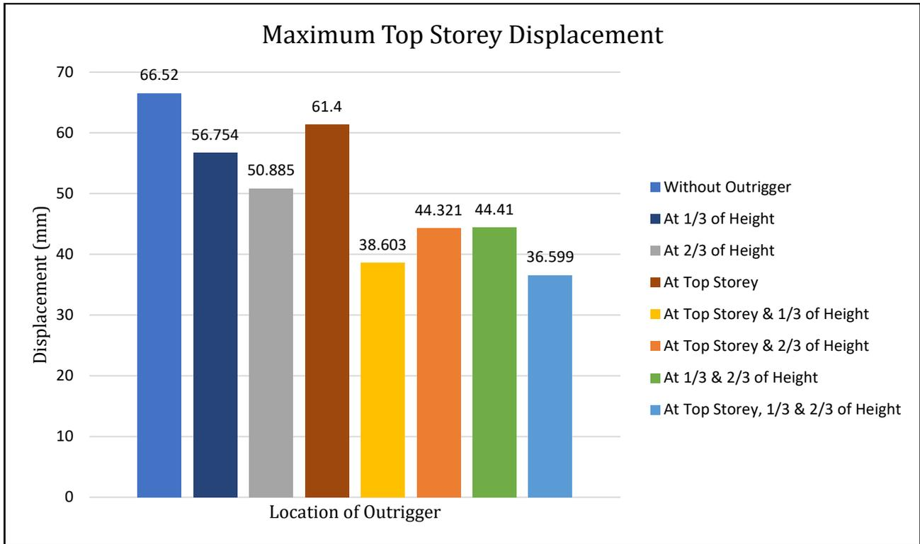
Figure 34 Maximum Top Story Displacement in RS-X & Y Direction (Response Spectrum)
