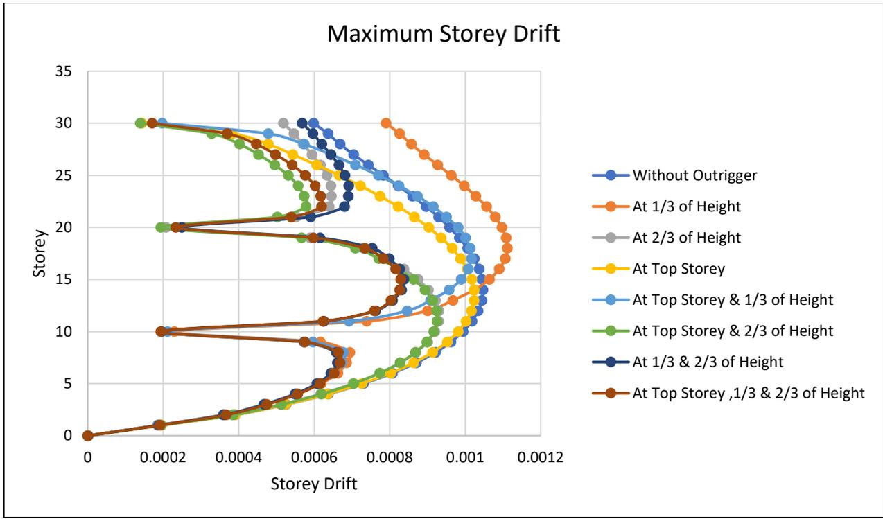
Figure 38 Maximum Storey Drift in EQ-X & Y Direction (Earthquake Static)
