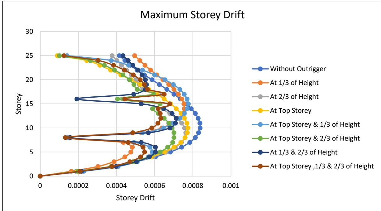
Figure 30 Maximum Storey Drift in RS-X & Y Direction (Response Spectrum)
