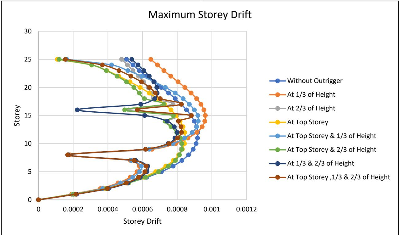
Figure 28 Maximum Storey Drift in EQ-X & Y Direction (Earthquake Static)
