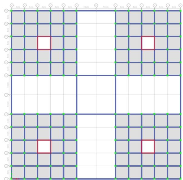
Figure 3 Typical floor plan of G+24 & G+29 Belt-truss building.
