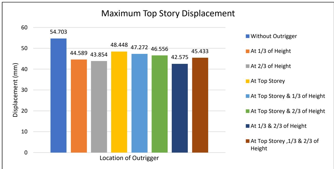
Figure 12 Maximum Top Story Displacement in EQ-X & Y (Earthquake Static)
