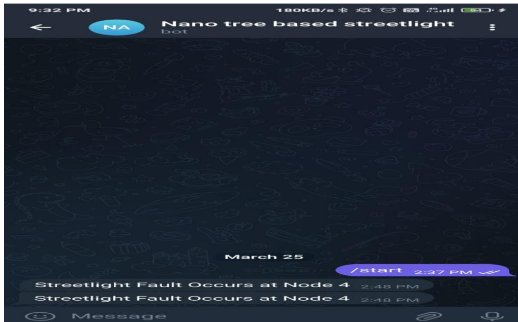
Fig. 4.5 Notifying on telegram physical damage of streetlight bulb stating 'Streetlight Fault Occurs at Node X'.
