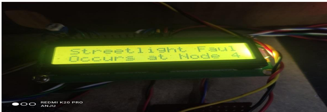
Fig. 4.4 Displaying on LCD 'Streetlight Fault Occurs at Node X'
