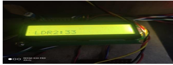
Fig. 4.3 Reading when streetlight's light not falling on LDR2
