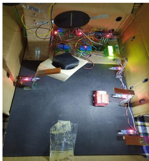
Fig. 4.2 Automatic Turn ON of streetlights at night and Intensity control
