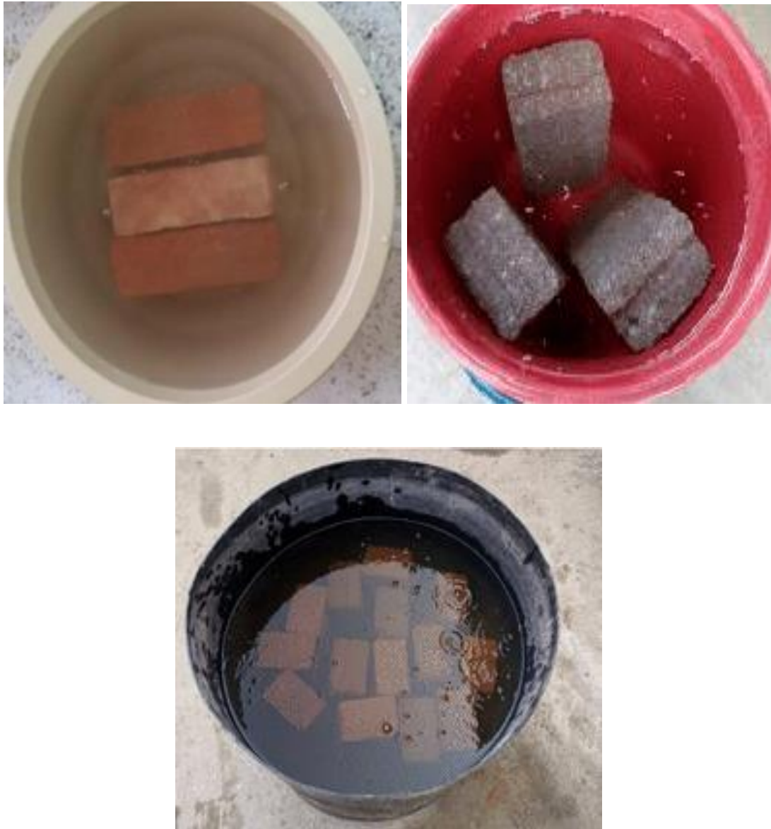
Fig 5: Water Absorption Test
