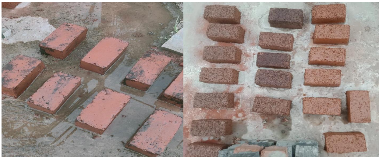
Fig 3. Laterite Soil Paving Blocks by Using Plastic
