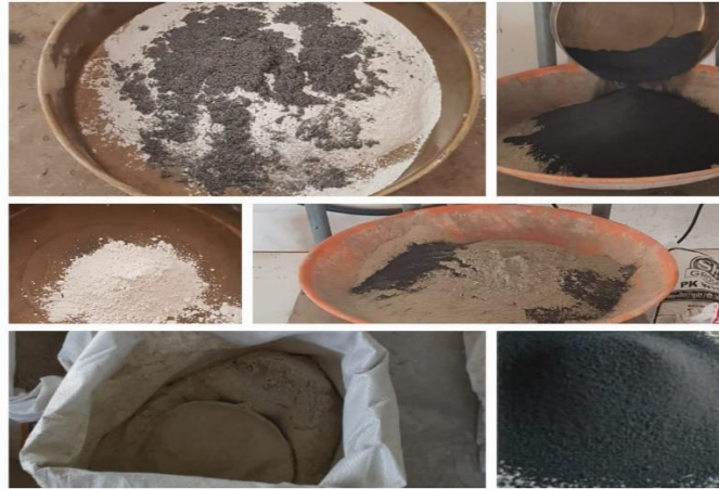
Figure1.1- Raw material used in AAC Block
