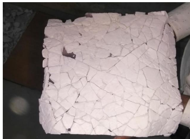
Figure : Breaking Pattern after Jolting test
