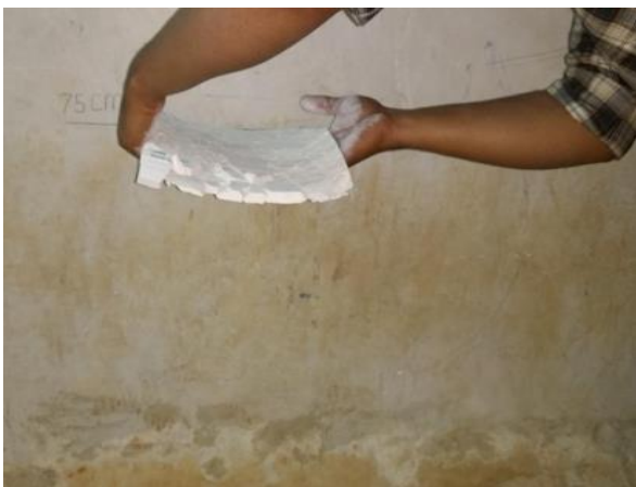
Figure : view of Jolting test showing HT 75 Cm
