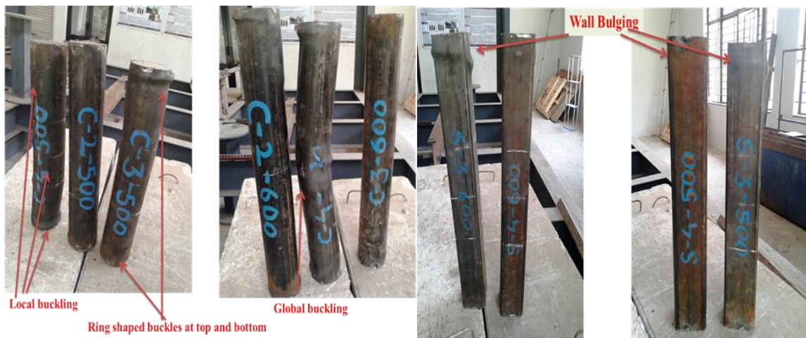
Fig.4.1: Failure modes for circular & square columns
