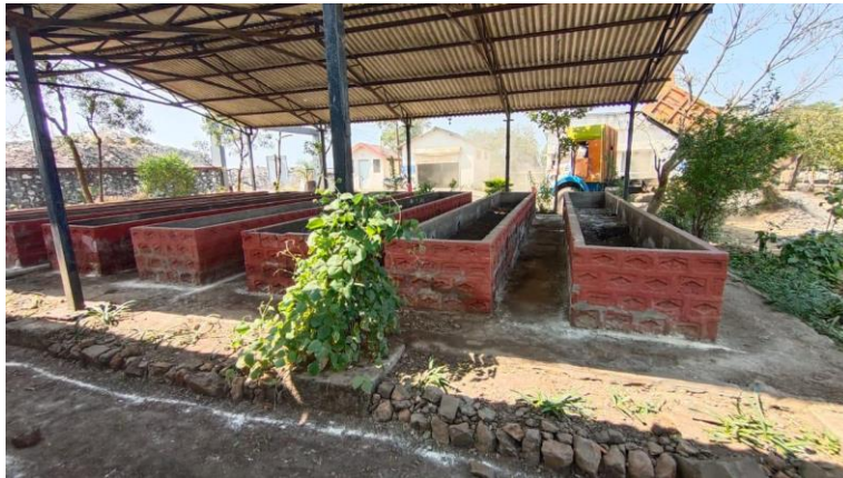
Fig. 3: Pit Composting in Kagal MSW plant (24ft x 3ft)
