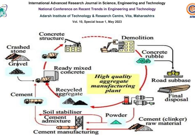
Quality of recycled aggregate and its concrete: The strength of recycled aggregate concrete is about 10 to 15 percent less as compared to concrete with fresh aggregate. However suitable mix designs may be made and reliable results obtained. The mix requires a slightly higher quantity of cement or using admixtures to reduce water requirement. Recycled aggregate concrete can be safely used as plain concrete. With proper corrections in mix design, it can be used for R.C.C. works also.
