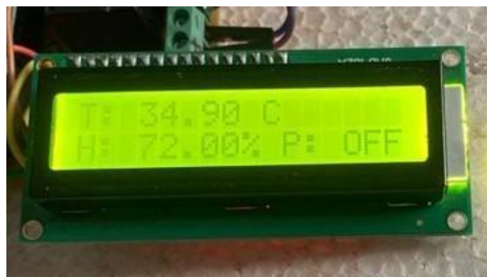
Fig 1. Hardware when mains power goes down.
