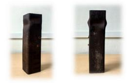
4. Square Rod 2 (Compression Test) Outer Side (a) = 49 mm Inner Side (b) = 43 mm A = 49<sup>2</sup> - 43<sup>2</sup> = 552 mm P = 149.6 KN = 149.6\*10<sup>3</sup> N ∴ σc = P/A = 149.6\*10<sup>3</sup> / 552 = 271.01 N/mm2
