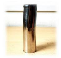
3. Square Rod 1 (Compression Test) Outer Side (a) = 39 mm Inner Side (b) = 34 mm  $A = 39^2 - 34^2 = 365 mm$   $P = 170.4 \text{ KN} = 170.4*10^3 \text{ N}$  $\therefore \sigma c = P/A = 170.4*10^3 / 365 = 466.85 \text{ N/mm2}$
