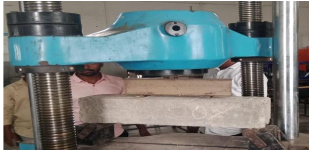
Fig 9: Flexural strength test on Beam.
