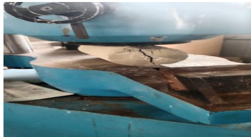
Fig 7: Split tensile strength test on Cylinder.
