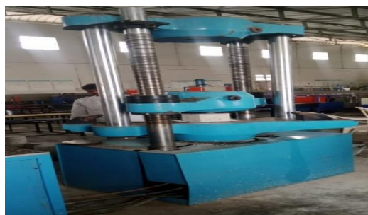
Fig 6: Compressive strength test on Cubes.
