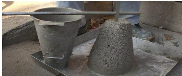
Fig 5: Slump cone test.
