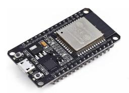
The ESP32 is a popular and widely used microcontroller module that integrates Wi-Fi and Bluetooth capabilities. Developed by Espressif Systems, the ESP32 is designed for a wide range of applications, including Internet of Things (IoT) devices, home automation, robotics, and more. Here is some information about the ESP32.
