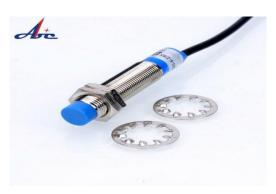
is a device that is used to detect the presence of metallic objects or materials in its vicinity. It operates on the principle of electromagnetic induction, utilizing a coil or antenna to generate an electromagnetic field and detect changes in that field caused by the presence of metal.
