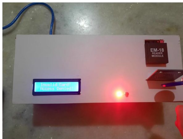
Figure 5: Output when an invalid tag is read
