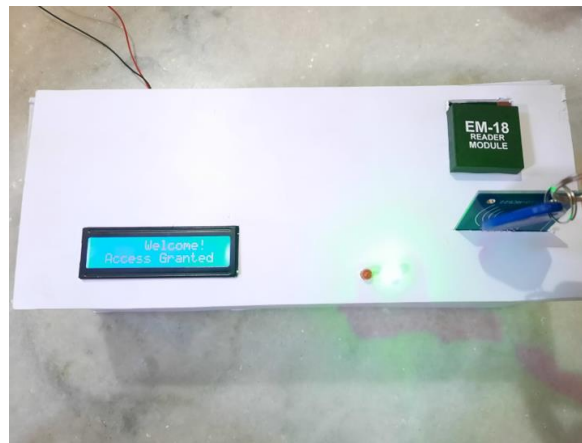
Figure 5: Output when a valid tag is read
