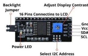
Fig - 5: I2C Module pin diagram
