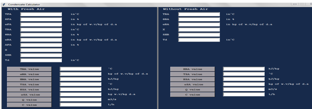
Figure 1 Screen shot of condensate calculator developed by using Python language
